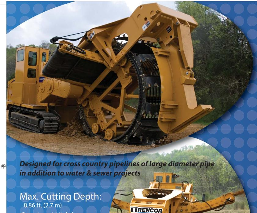
Rotary Surface Mining attachment ...transforms a heavy-duty Trencor chain trencher into a high performance excavator that cuts through rock in a consistent, single pass at a controlled grade
