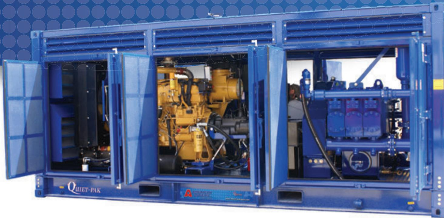
American Augers mud pumps are stand-alone, self-powered machines. They are ideal accessories with mud motors, large reamers or wherever mud volume is needed downhole.
