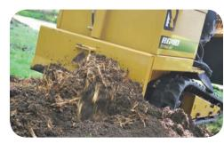
Hydraulic Backfill Blade Standard
