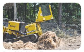
Standard Hydraulic Backfill Blade
