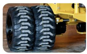
Dual Rear Wheels for Increased Stability and Traction
