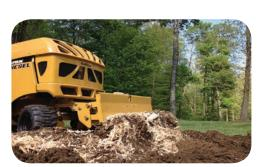
Hydraulic Backfill Blade
