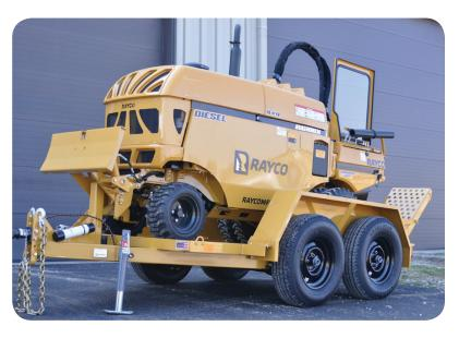
The RAYCO TR100 trailer is specifically designed to haul the RAYCO RG45T, RG70X (RG70XR), and RG100X (RG100XR) self-propelled stump cutters. The TR100 features a single-pin lock to secure the stump cutter to the trailer. Standard features include: electrostatic powder-coat paint, skid-resistant deck and ramps, electric brakes and tandem Dexter E-Z Lube leaf spring suspension axles.
