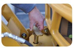
Single Pin Lock to Secure Stump Cutter to Trailer
