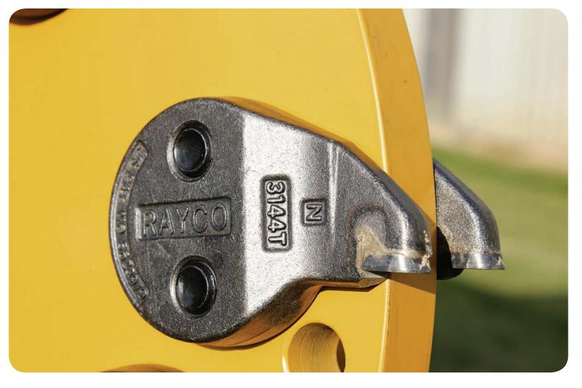
The Rayco Super Tooth can maximize the cutting performance of almost any stump cutter, including competitive brands. This time tested design incorporates the mounting block, neck, and strike point into one massive cutting tool. Unlike other tooth designs, the Super Tooth has extra mass in the neck to eliminate bending, twisting, and breaking that can cause machine shut down and high maintenance costs. It also increases cutter wheel thrust, balance, and inertia
