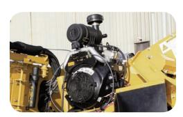
40hp Subaru Gasoline Engine
