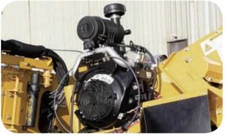
40hp Subaru Gasoline Engine
