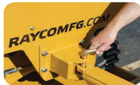
Single Pin Lock to Secure Stump Cutter to Trailer
