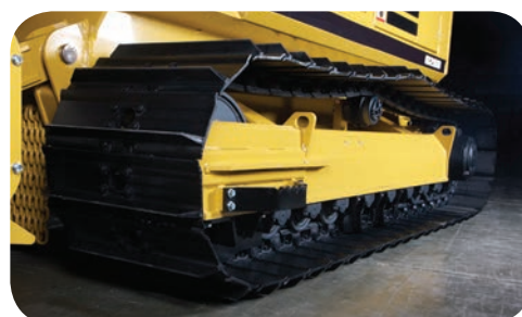
Heavy Duty Undercarriage with 2-Speed Final Drives
