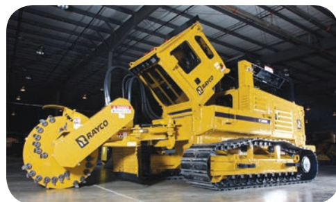
Tilt Cab for Access to Hydraulic Components
