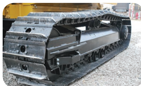
Heavy Duty Undercarriage with 2-Speed Drives
