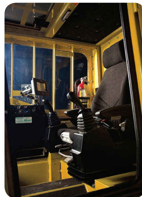
Forestry Cab with Rooftop Escape Hatch and Heated, Suspension Seat
