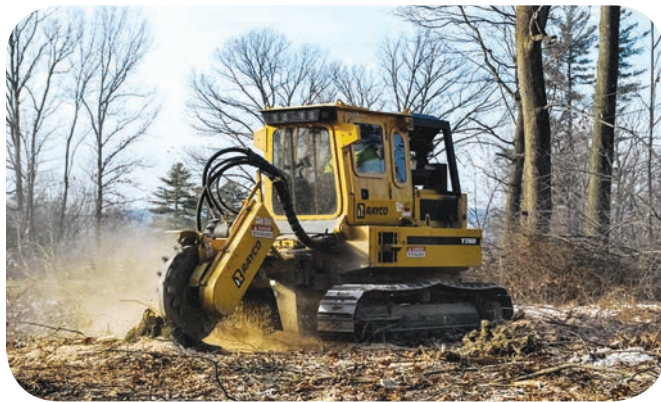
Powered by 260 Hp Cummins 6.7L Turbo Diesel
