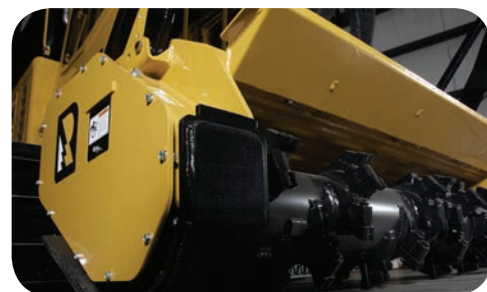
Predator Mulcher with Dual Variable Displacement Motors
