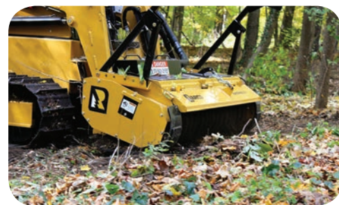
Predator Mulcher Head with Variable Displacement Motor
