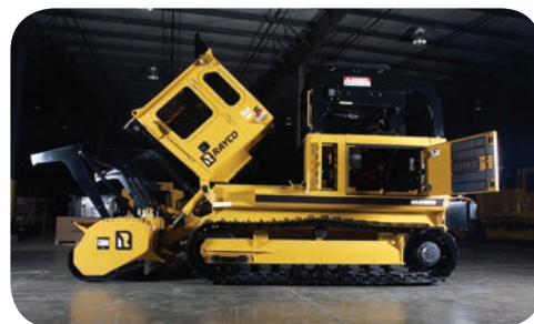
Hydraulic Tilt Cab For Easy Access to Engine and Hydraulic Components
