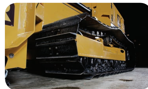
Heavy Duty Steel Undercarriage with 2-Speed Final Drives
