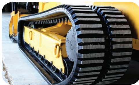
Rubber Track Undercarriage with 2-Speed Travel
