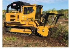
102 gpm cutter system provides hydraulic power to 7-foot Predator mulcher head.
