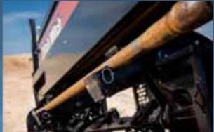
2 Add-a-pipe feature places individual pipes into loading system without lifting pipe into the top of the pipe box
